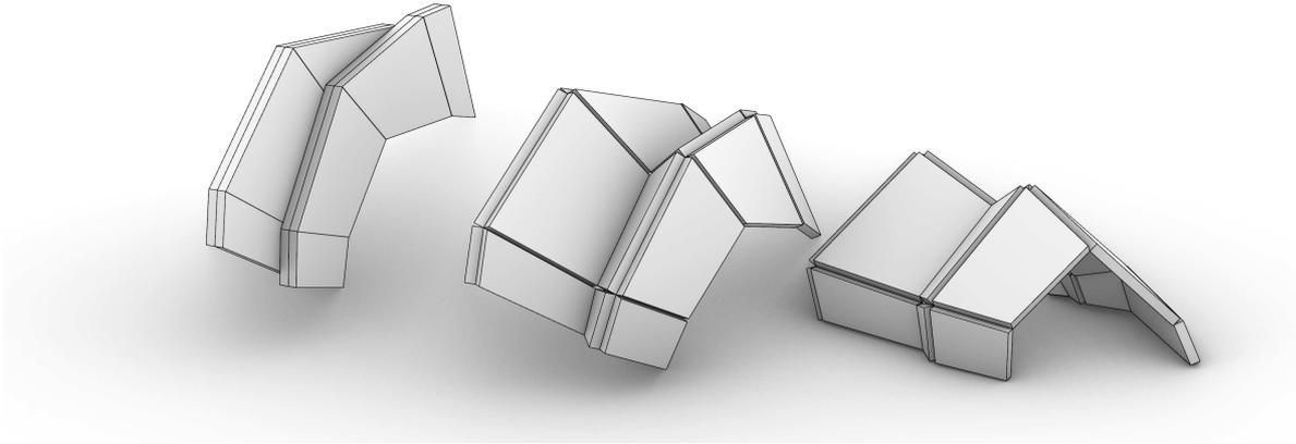
**Figure 13:** Folding motion of a freeform bellow-type structure composed of  $4 \times 4$  panels using 2 types of thicknesses.
