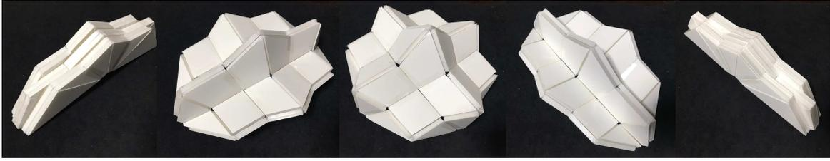
**Figure 20:** Folding motion of the bidirectional flat-foldable model. Thickness a: 7mm, b: 8mm (assumed that standard dimensions of 21-mm and 24-mm thickness is used.)
