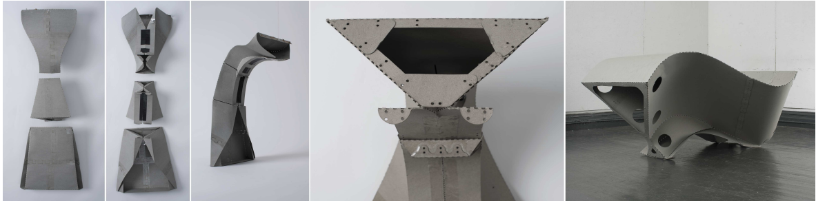
Figure 8: Three sub-assemblies of a column, planar joint, 2.5m large prototype.
