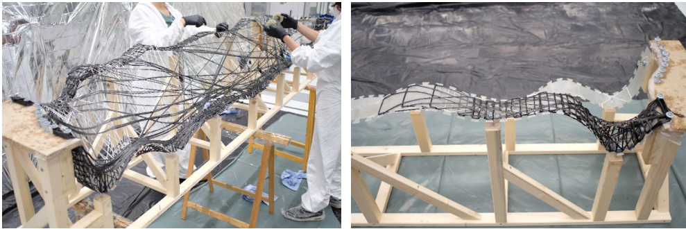
Figure 16: (a) Image during the winding of a crease, (b) Image of the winding of the infill surface [images by the authors].
