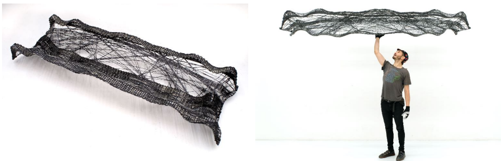
Figure 20: Physical prototype of a Filigree Shell Slab component: (a) Top view, (b) Side view.
