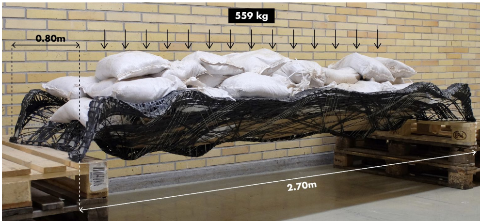
Figure 21: Load testing the prototype.
