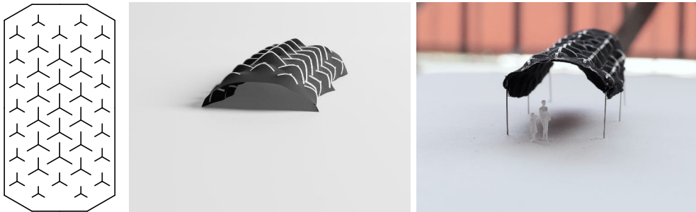
Figure 1: Our printing-on-fabric meta-material encodes surface curvature within a regular star pattern (left). Our predictive simulation allows the virtual design of architectural models (middle), with a close match to physical realization (right).
