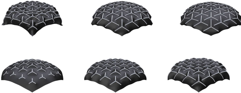
Figure 8: We show the effect of two design parameters on the equilibrium shape of the star meta-material: the length of the star arms \ell and their thickness h . For this experiment we print 37 stars on a hexagon of fabric with side length 67 mm. In the top row we fixed \ell = 10 mm and set, from left to right, h with a decreasing radial gradient from 0.6 mm to 0.2 mm, a constant value of 0.4 mm and an increasing gradient from 0.2 to 0.6 mm. In the bottom row we fix h = 0.3 mm and prescribe three different radial gradients for \ell : a decreasing gradient from 10 mm to 4 mm, and constant value of 7 mm and an increasing gradient from 4 mm to 10 mm.
