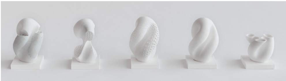
Figure 13: Strategies to adjust the flexibility of the connections by: (a) creating two parts out of a stiff core and soft grips, (b) interlocking detail of the two part connection, (c) differentiated perforation on the surface (d) adjusting the infill structure and (e) creating a hollow core. Photo credits: Julius Hatt.
