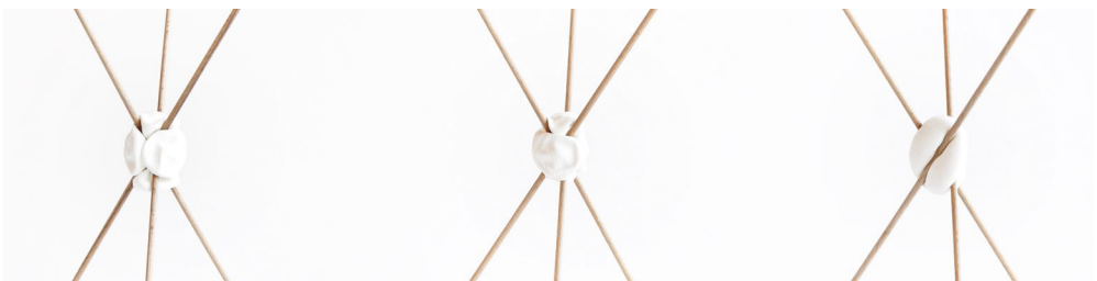
Figure 11: Fabricated models of studies with primitive geometries outside the bundling (a),(b) and in between the members (c). Photo credits: Julius Hatt.
