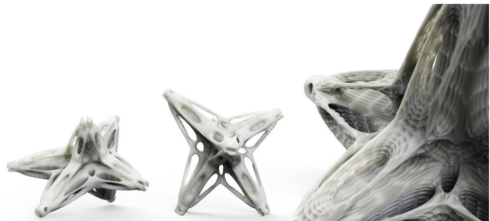
Figure 19: Close preview of an ornamented joint with two levels of subdivision to articulate the surface.
