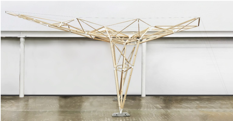
Figure 23: The canopy in numbers: 47 bespoke 3D printed nodes, 157 members, 600 screws. Max. height 3 m , width 2.7 m, and cantilever 4 m. Photo credits: Alexander Enz.
