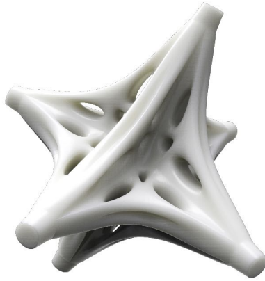
Figure 16: Stiff connection with complex topology created with MOLA (Dillenburger et al. 2019) open-source pure python mesh library and subdivided with customized rules".
