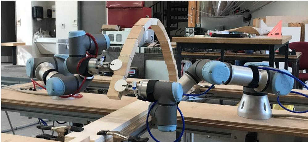
**Figure 9:** Small-scale prototype to test the alternating placement strategy for a brick arch with a running bond pattern.
