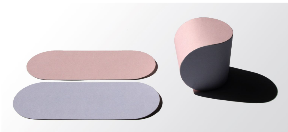
Figure 7: Elementary dForm and cutting patterns consisting of half-circles and line segments.
