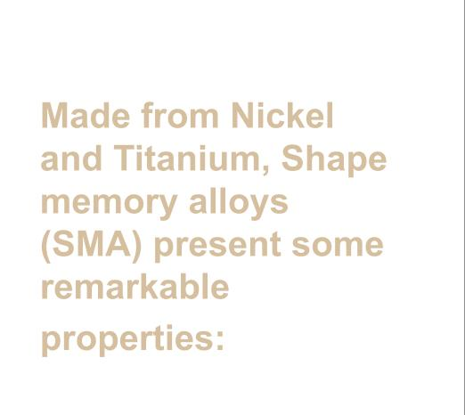
**Thermomechanical properties:** This so-called "smart material" can undergo large deformations (up to 8%) and return to its original shape with a high recovery force when heated, which is known as the "shape-memory effect." This feature relies on a solid-solid phase change at the crystal lattice level resulting in a coupling between temperature and mechanical loads.
